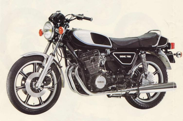
Three cylinders, double overhead camshafts, 747 cc, shaft drive and setting new standards in braking, handling and overall design. The all-new Yamaha XS750 proves that not only is it the worlds latest superbike but that it MUST lead in its class. The cast alloy wheels fitted as standard equipment with a double disc brake on the the 19 inch front wheel and a single disc on the 18 inch rear, acknowledge the expe-
