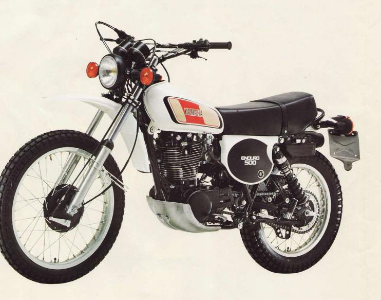
Yamaha's XT500 Enduro is a bike with real character. And it's unique. The 499-cc, single cylinder, overhead-cam engine brings back the delights of the big single "Thumper" to the world of motorcycling.
