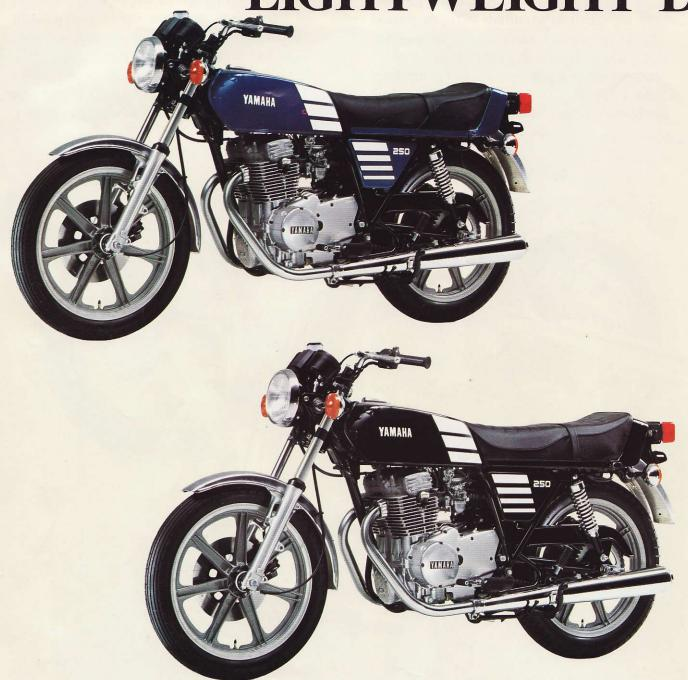
A new two-fifty star has land on earth! The XS250 is a dream package that holds every element of exciting motorcycling. A 4-stroke single-overhead-camshaft, twin cylinder engine powers an economical, six-speed machine, which with its cast alloy wheels, complete luxury specification and scintillating performance, will capture top billing in any motorcycle scene where a two-fifty is considered ideal. This smooth
