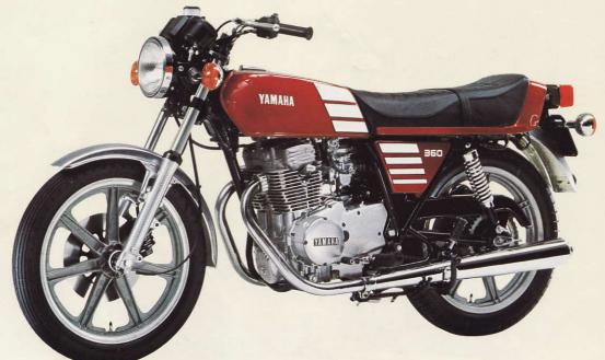
The XS360 is not just a new Yamaha Motorcycle, it is the world's best quality middleweight contender. Take the 180-degree crankshaft layout for vibration-free, twin-cylinder running. Add the best electrical components of almost any machine on the market, such as a three-phase, electromagnetic field coil system that keeps the battery fully charged even on short runs or stop-go-in-town-work. Further consider the refinements of an automatic fuel tap and a single adjustment screw to synchro-
