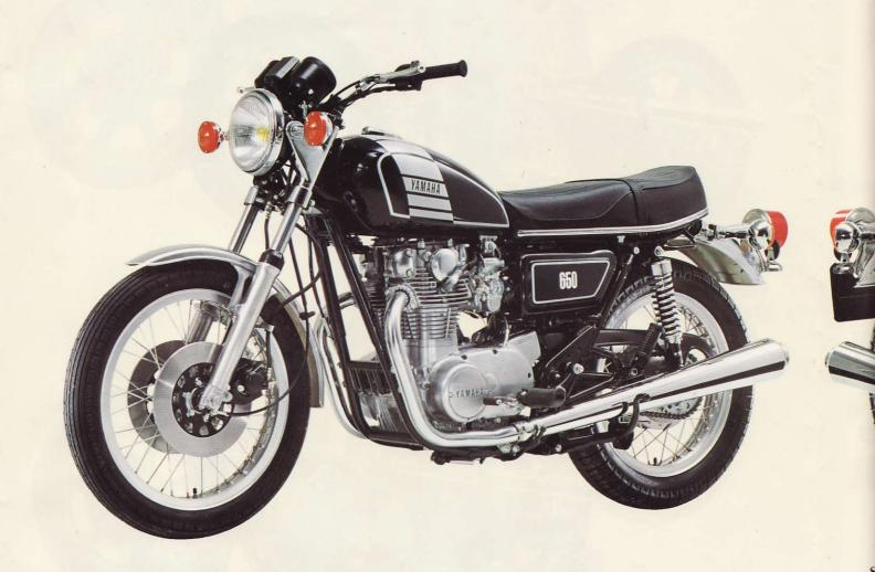
The first Yamaha 4-stroke machine was a 650 and it became market leader in its class. Today refined and improved the XS650 is a unique class machine proving that the traditionalist still wants 50 hp six-fifties for everyday use. The XS650 is powered by a 653cc parallel-twin engine with valves operated by a single, chaindriven, overhead camshaft. A technical breakdown of this 650 reveals a bore and
