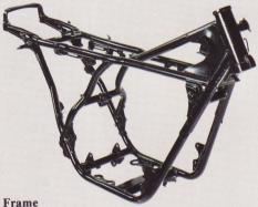
In order to give the bike better dynamic stability, the high-tensile-strength, double-cradle frame carries the engine low and forward. This tubular-steel frame is also designed to be able to withstand twisting, turning and impact stresses that are incurred on the roughest of roads so that the bike will be able to offer dependability regardless of the road conditions.
