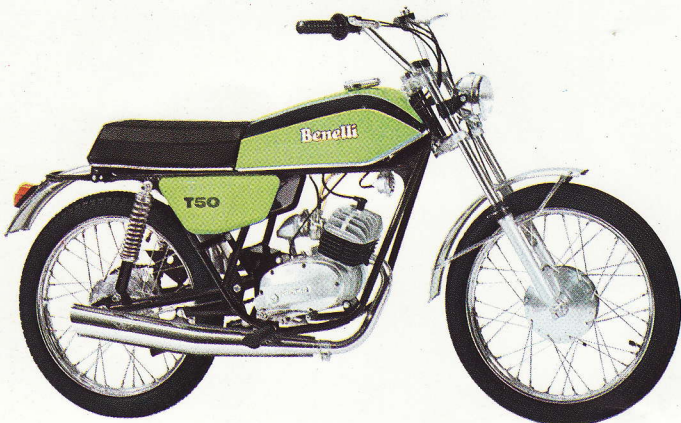
50 TURISMO • Engine 2 stroke – single cylinder 49 cc – gear box 5 speed with foot control lever – 2.50x18" wheels – dry
