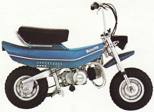
CADDY • Engine 2 stroke – single cylinder 49 cc – single speed – automatic centrifuge clutch – 3.50x7" wheels – dry weight Kg. 42
