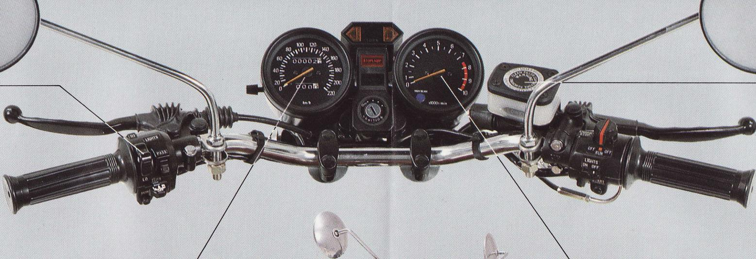
Fluid reservoir for twin front disc brakes is on the right handlebar grip. Bell-crank levers give extra leverage. On the twistgrip bars are engine cut-out switch, lights switch and electric starter button.
